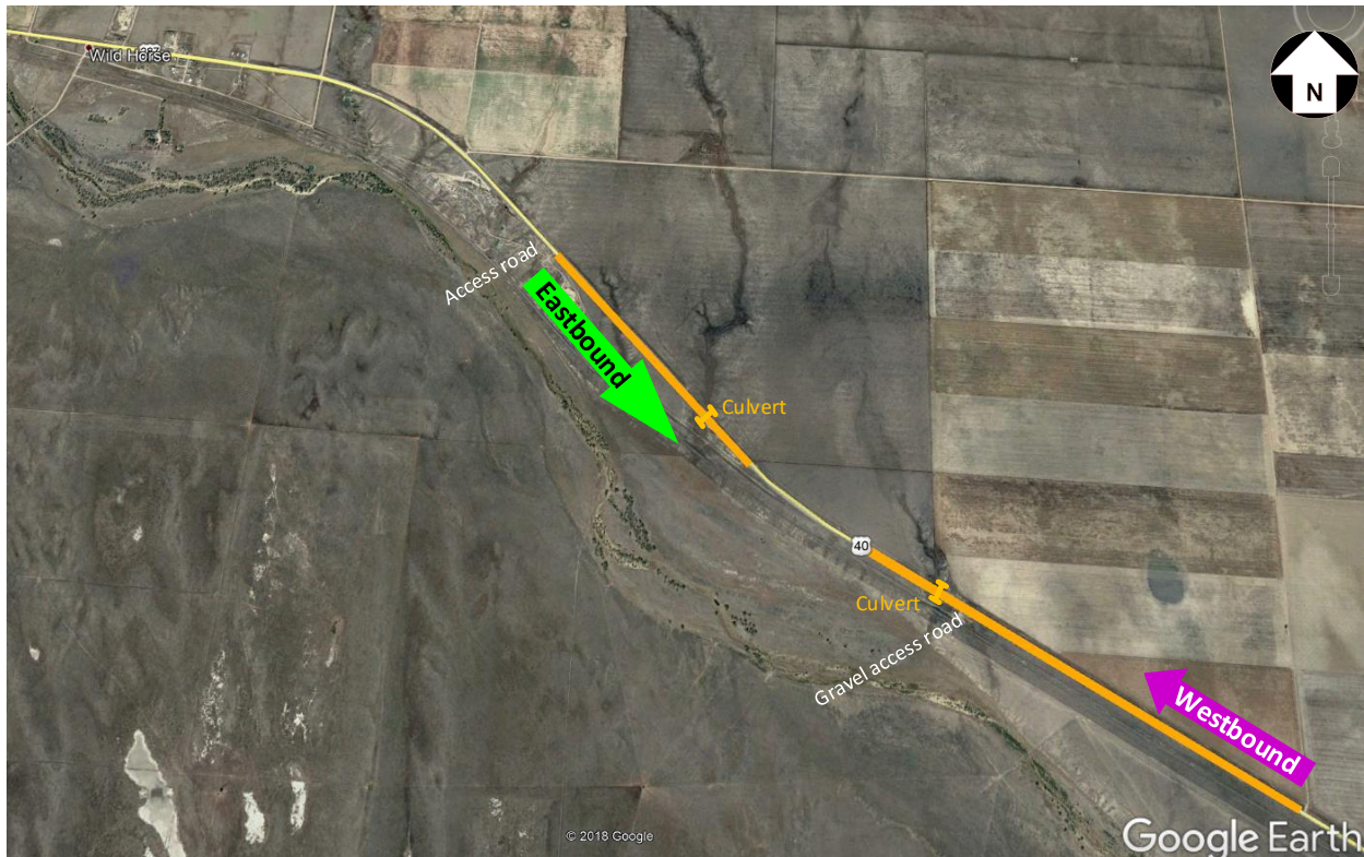
Figure 11: Alternative Passing Lane Locations on Westbound US 40
